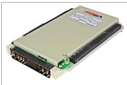
Figure 1 | Behlman's 3U COTS VPXtra 500M card is designed for use in airborne, shipboard, vehicle, and mobile applications.
