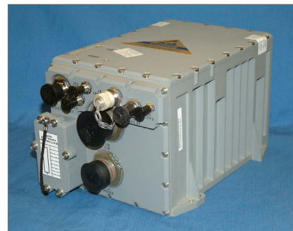
Figure 1 | Pictured is Honeywell’s EGI FALCN navigation system, launched this year. It is a smaller, lighter version of the company’s H-764, for defense aircraft.
