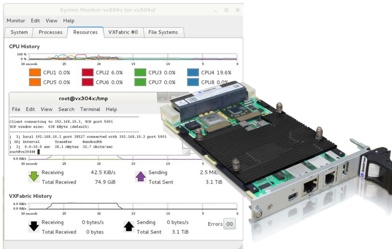
Figure 1 | Kontron VXFabric supplies the needed software between the PCIe Gen 3 switch and the bottom of the standard TCP/IP stack to enable boards to run any existing TCP/IP-based application without having to be modified. This interconnect fabric resource simplifies and helps propel application development of inter-CPU communication in VPX system architectures, enabling military OEMs to reduce development costs.
