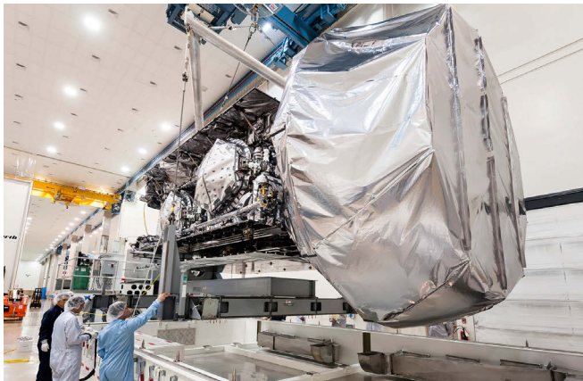
Figure 1 | Lockheed Martin engineers prepare to ship the third MUOS satellite to Cape Canaveral Air Force Station in Florida. Photo courtesy of Lockheed Martin.
